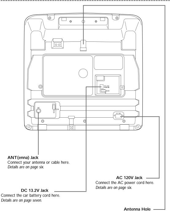
Connect the base stem of the supplied rod antenna here. Details are on page six.
